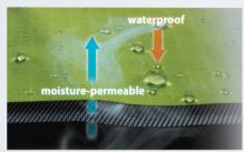
Moisture-permeable, waterproof fabric water scarcely permeate even the water-resistant pressure of 1,000mm ■DFJ212 ■DFV210
