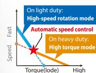
Automatic torque Drive Technology (ADT) adjusts speed and torque during operation for optimum performance
